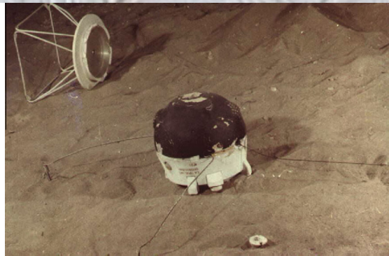
Fig. 5. Phobos Hopper qualification model after test (courtesy: VNIITransmash).
