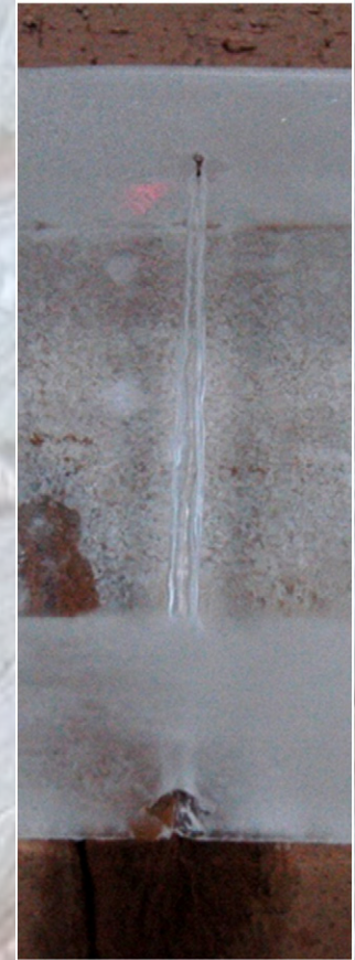
Fig. 3. Ice block penetrated by CO 2 laser irradiation. The laser entered from top picture. The hole diameter is about 4 mm and the hole length is about 13 cm is under the ice block in the front.
