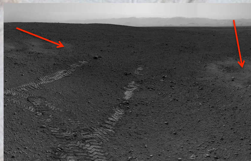
Images of Curiosity landing site where is possible to see the erosion effect of sky-crane thrusters,
