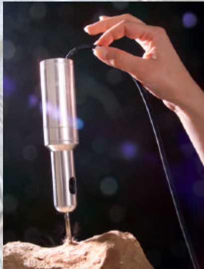
Fig. 1. A photographic view of the USDC held from its cable while coring sandstone. The minimal need for axial force is easily seen.
